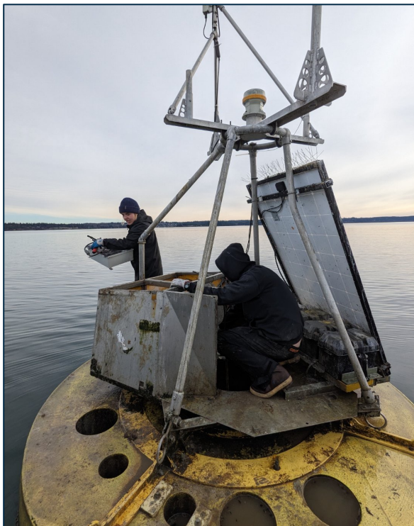
An ORCA buoy 15 years later in 2023, with years of grime, corrosion, and bird poop.
